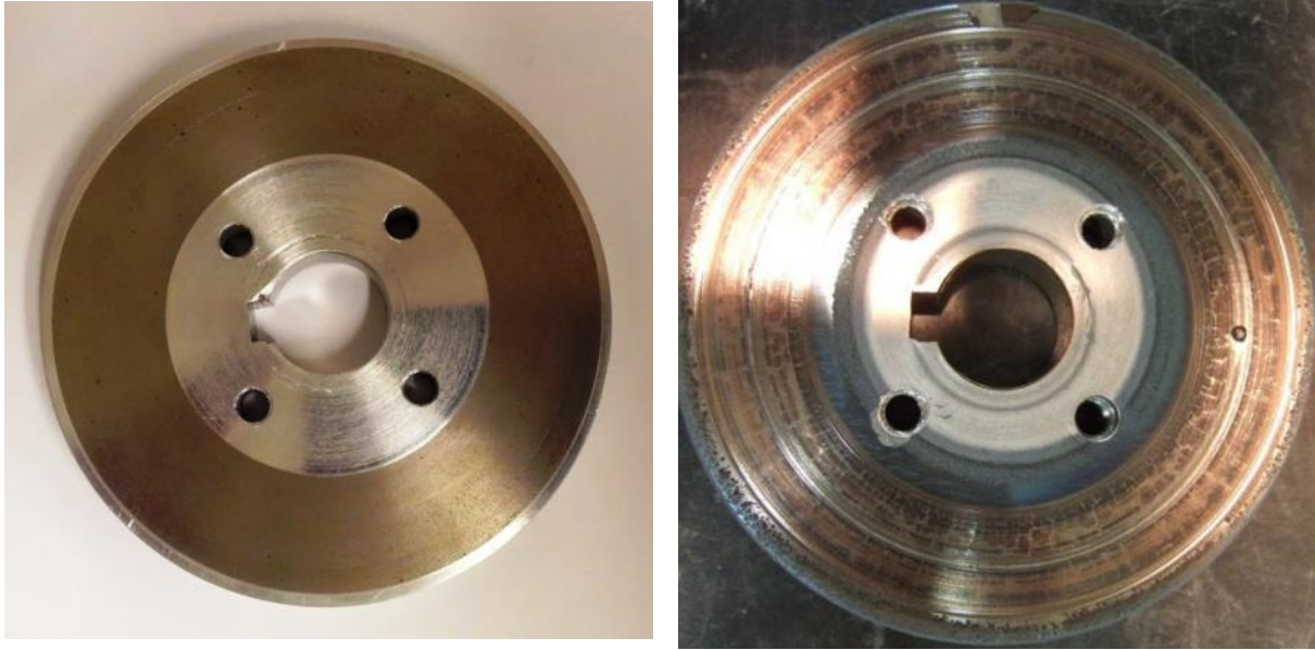
Figure 8.4: Aluminum pucks with cold sprayed Fe-Mn 2 coatings before and after testing
