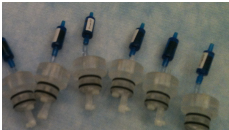
Fig. 6 Check valves on third iTIE cap port to provide air vent for organism chamber. These were tested as a method to prevent air bubble formation that could stop water flow through the 2004 Burton/Nordstrom system.
