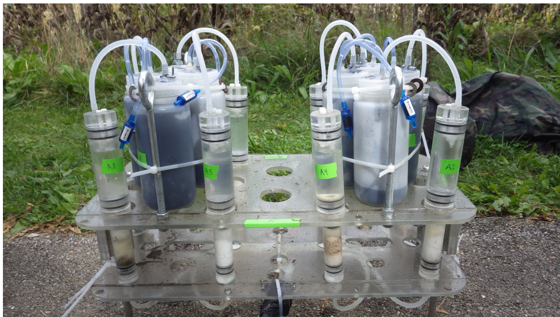
Fig. 14 iTIE Field Version II (Complete). This version was used for the three WERF field studies as an in situ TIE prototype.
