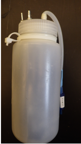
Fig. 10 Field Version II Sample Collection Bottle (left) and cap with flow valve and outflow port (right)
