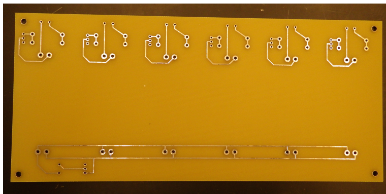
Fig. 31 Printed circuit board without circuitry components. This board, its components, and the battery constitute the flow control mechanisms for iTIE Version III. Pump power and speed is controlled with power switches and voltage regulators (not pictured).
