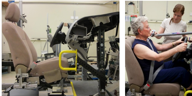
(b) driver mockup and recording body landmark locations using a FARO Arm coordinate digitizer
