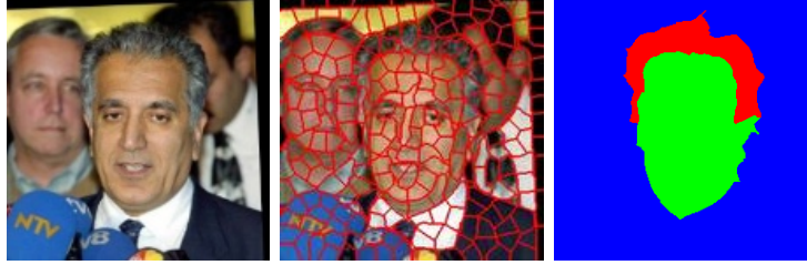
Figure 5.1: The left image shows a “funneled” or aligned LFW image. The center image shows the superpixel version of the image which is used as a basis for the labeling. The right image shows the ground truth labeling. Red represents hair, green represents skin, and the blue represents background.
