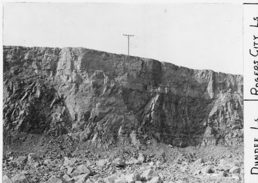
FIGURE 2. VIEW OF PART OF SOUTHERN FACE OF MICHIGAN LIMESTONE AND CHEMICAL COMPANY QUARRY AT ROGERS CITY, SHOWING CONTACT OF THE DUNDEE AND ROGERS CITY LIMESTONES. Light band just above contact represents the conspicuous dolomite described as interval 5 of quarry section (p. 10).
