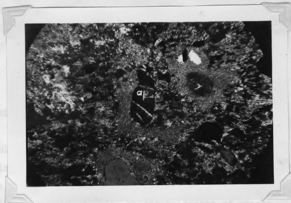
A. Boulder Creek granite next to the vein, Cold Spring mine, new shaft, 5th level. Nicols crossed. X65.
