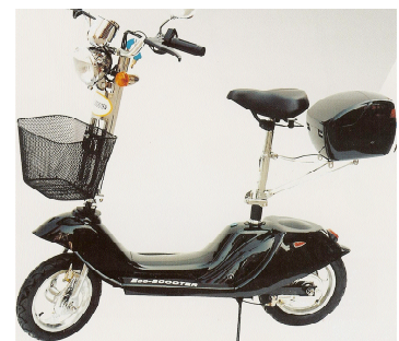
Modern Bug YT904 250W/24V/12Ah 24kph/20km Zhejiang Yeying EPowerV Co
