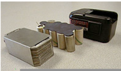
EEI NiMH bipolar (left) power tool NiCd pack (right)
