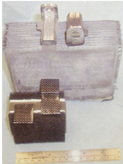
Lead-Acid Plates and Firefly Carbon Foam
