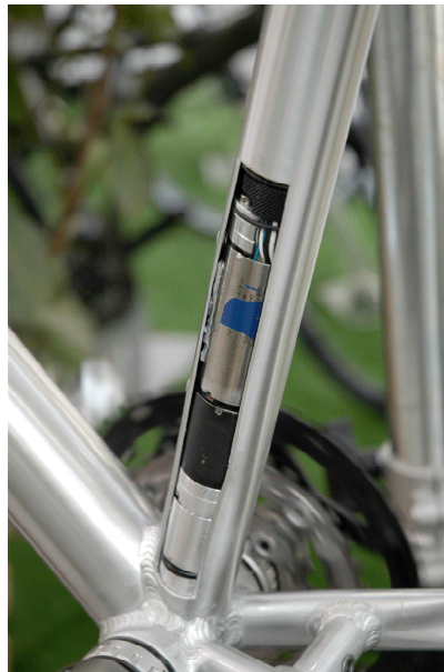
Gruber - motor in down tube
