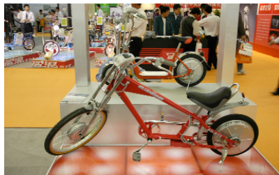
Battery in the rear wheel
