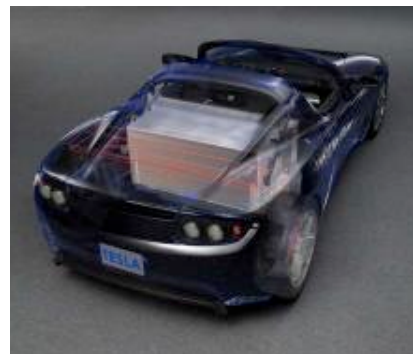
Tesla Battery Location
