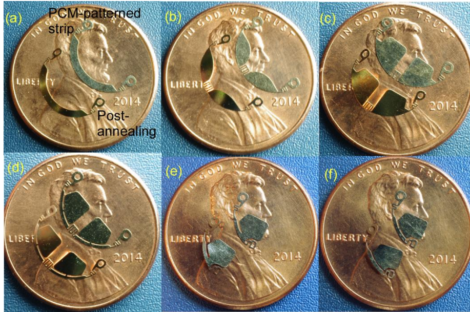
Fig. 3.6: Fabricated actuators after photochemical machining and annealing: (a) Type A, (b) Type B1, (c) Type B2, (d) Type C, (e) Type D1, and (f) Type D2.
