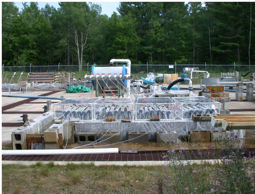
Fig. 12. Experimental streams built at the UMBS Artificial Stream Laboratory, where water can be pumped out of the East Branch of the Maple River to a concrete pad and distributed into artificial streams.
