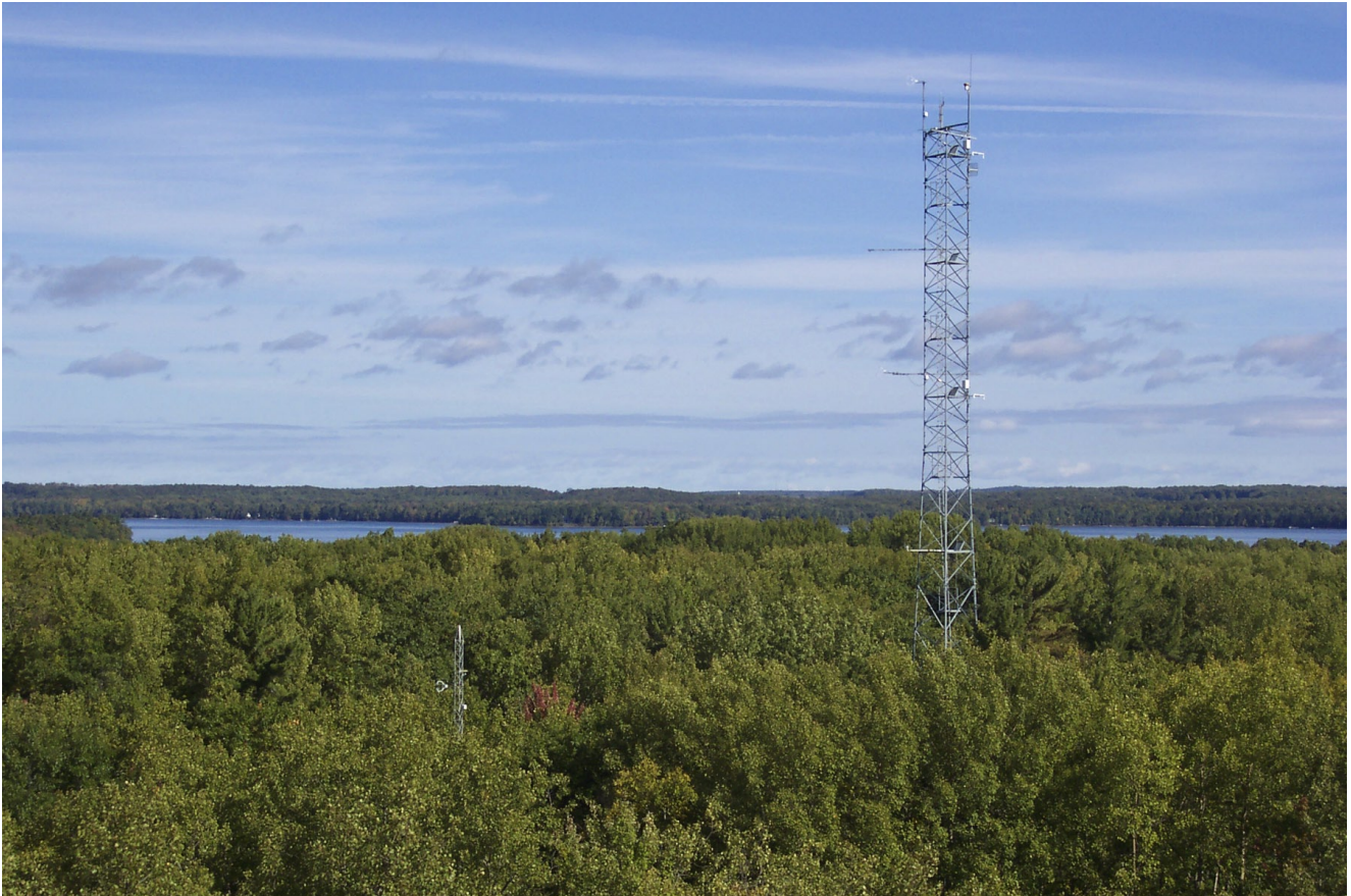
Fig. 9. The 50-m Ameriflux tower, with Douglas Lake in the background. This photograph was taken from the 35-m Prophet tower. Both towers are equipped with sensors for monitoring forest–atmosphere gas exchanges
