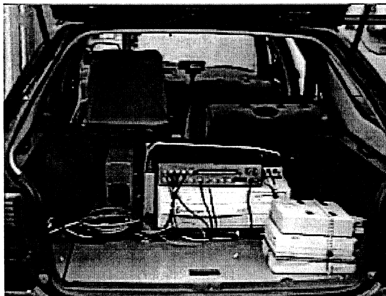
Figure 2. Data collection equipment and power supplies.
