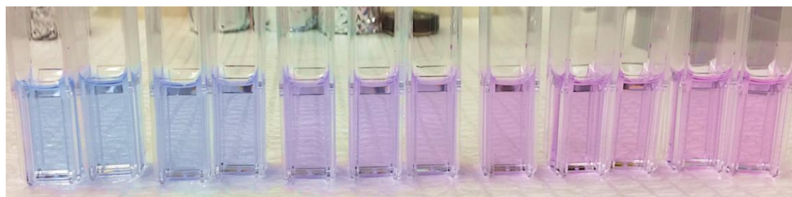
Figure 4. Color gradient of sodium ion sensors in [\text{Na}^+] of 0, 0.1, 0.5, 1, 5, 10, 20, 50, 100, 150, 200, and 500 mM.
