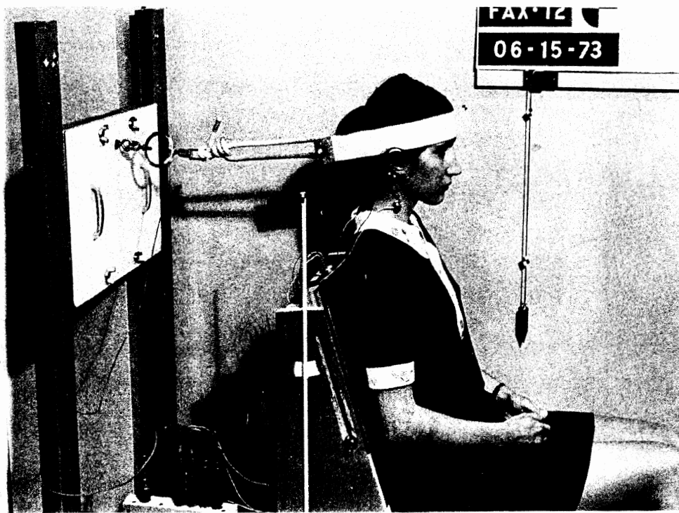
Figure 2-17. Measurement of flexor muscle isometric strength. Subject is seated in normal position. Electrodes recorded the EMG, and the force ring behind the subject measured muscle force.
