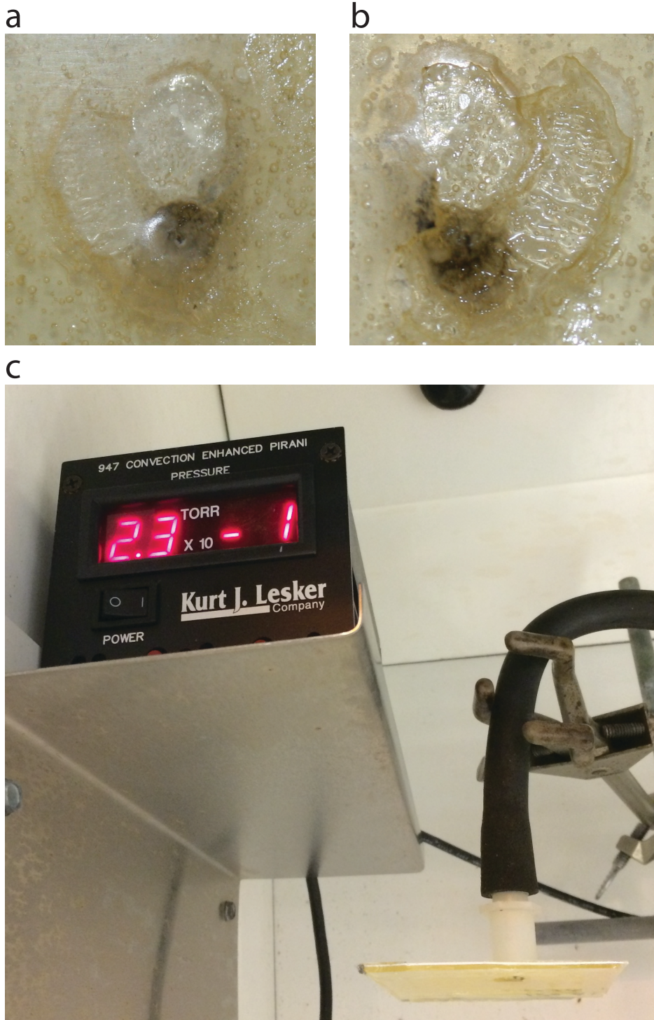
Figure 9: Photographs of a healed panel. a) Entrance- and b) exit-side photographs of a healed puncture site with the rear EMAA layer removed. c) Vacuum applied to entrance-side puncture site of this test panel with the EMAA layer removed. Note the vacuum gauge shows a vacuum of 2.3 \times 10^{-1} Torr, corresponding to a \Delta P across the polymerized thiol-ene plug of \sim 0.999 atm.
