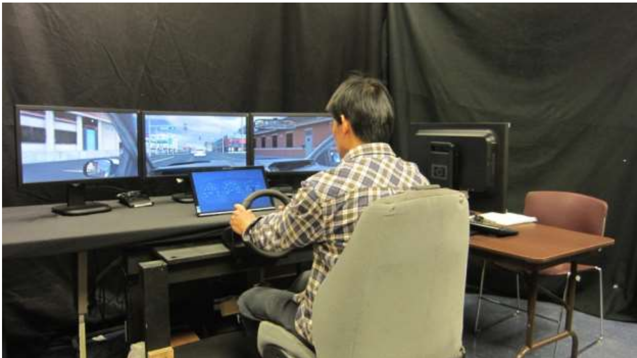
Figure 3. Driving Simulator Set-up
