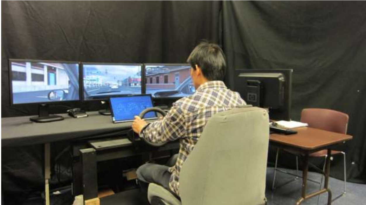
NADS MiniSim-based driving simulator with steering wheel and foot pedals
