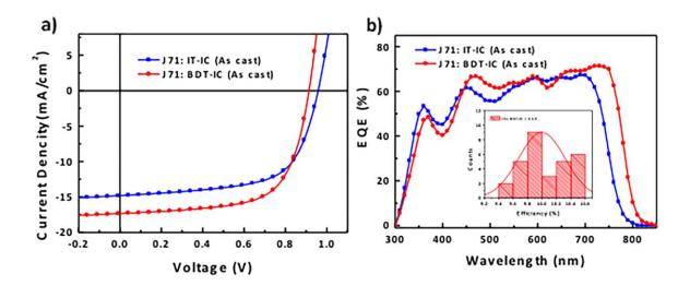
**Figure 3.** (a) Current-density-voltage characteristics, and (b) External quantum efficiency (*EQE*) spectra of the organic photovoltaic cells based on J71: IT-IC (1:1, w/w) and J71: BDT-IC (1:1.2, w/w). *Inset*: Histogram of efficiencies of organic photovoltaic cells (among 30 devices) based on J71: BDT-IC (1:1.2, w/w).
