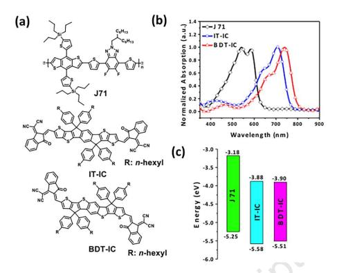
**Figure 1.** (a) Molecular structural formulae of J71, IT-IC and BDT-IC; (b) Normalized UV-Vis absorption spectra of J71, IT-IC and BDT-IC thin films; (c) Energy diagram of J71, IT-IC and BDT-IC relative to vacuum obtained from cyclic voltammetry measurements.
