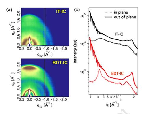
**Figure 2.** (a) Grazing incidence x-ray diffraction (GIXD) patterns of as-cast IT-IC and BDT-IC films; (b) In-plane (dotted line) and out-of-plane (solid line) x-ray scattering patterns extracted from the 2D GIXD images. Here, q is the scattering vector,  $q_{xy}$  is the in-plane direction and  $q_z$  is the out-of-plane direction.
