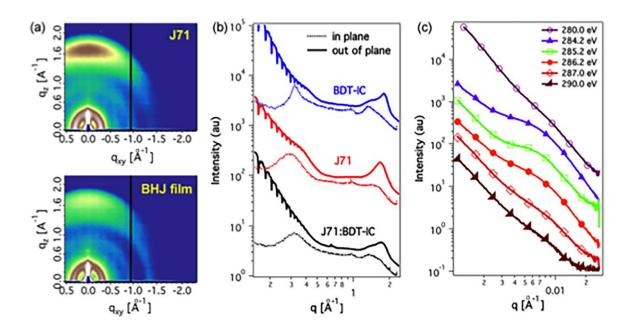
**Figure 5.** (a) Grazing incidence x-ray diffraction patterns; (b) patterns taken along the lines in (a), and (c) resonant soft x-ray scattering of J71, BDT-IC and J71:BDT-IC blends Here, q is the scattering vector,  $q_{xy}$  is the in plane direction and  $q_z$  is the out of plane direction.
