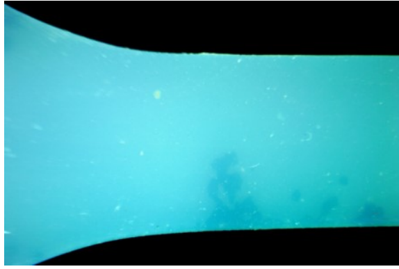
Figure 3.5: Stamped baseline specimen from a cast sheet of material. Spots are from dust particles.
