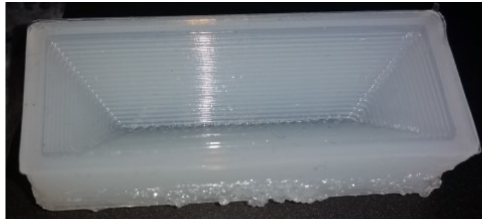
Figure 2.12: Bottom view of the bridging in Exp. IV Test 5 specimen.
