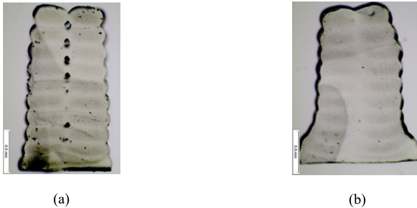
Figure 2.9: Cross-section of the double-line wall with (a) X = 1.02 and c_{edge} = 0.48 mm with voids and (b) X = 1.16 and c_{edge} = 0.42 mm with no void and taper at the base (initial layers).
