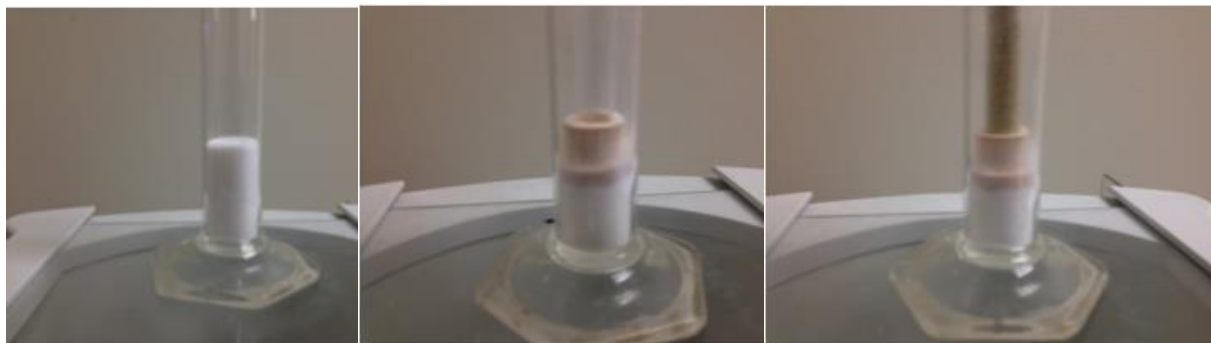
Figure 5. Efforts to compress gel 7. a. uncompressed density 0.06 g/mL, 719 mg powder fills 10 mL b. Density under a 5 g wt. = 0.12 g/mL (719 mg powder in 5.8 mL) c. Density under 300 g wt (9 kPa), 0.15 g/mL 719 mg powder in 4.9 mL.
