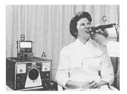
Fig. 5. Thermo-electric tooth stimulator system: (a) D. C. power supply. (b) Tele-thermometer. (c) Thermo-electric tooth stimulator.
