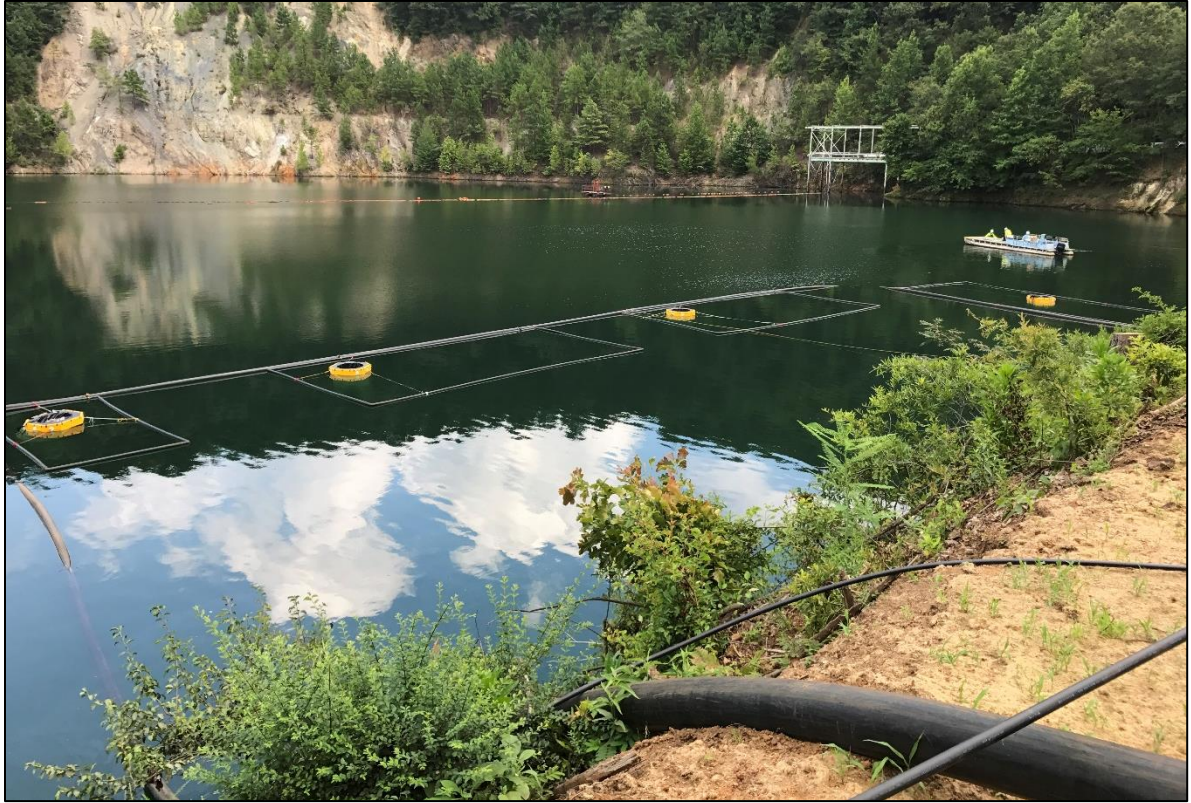
Figure B-3: Limnocorral placement within each test plot. From left to right: non-capped (control), Aquablok, limestone-bone char, and limestone.
