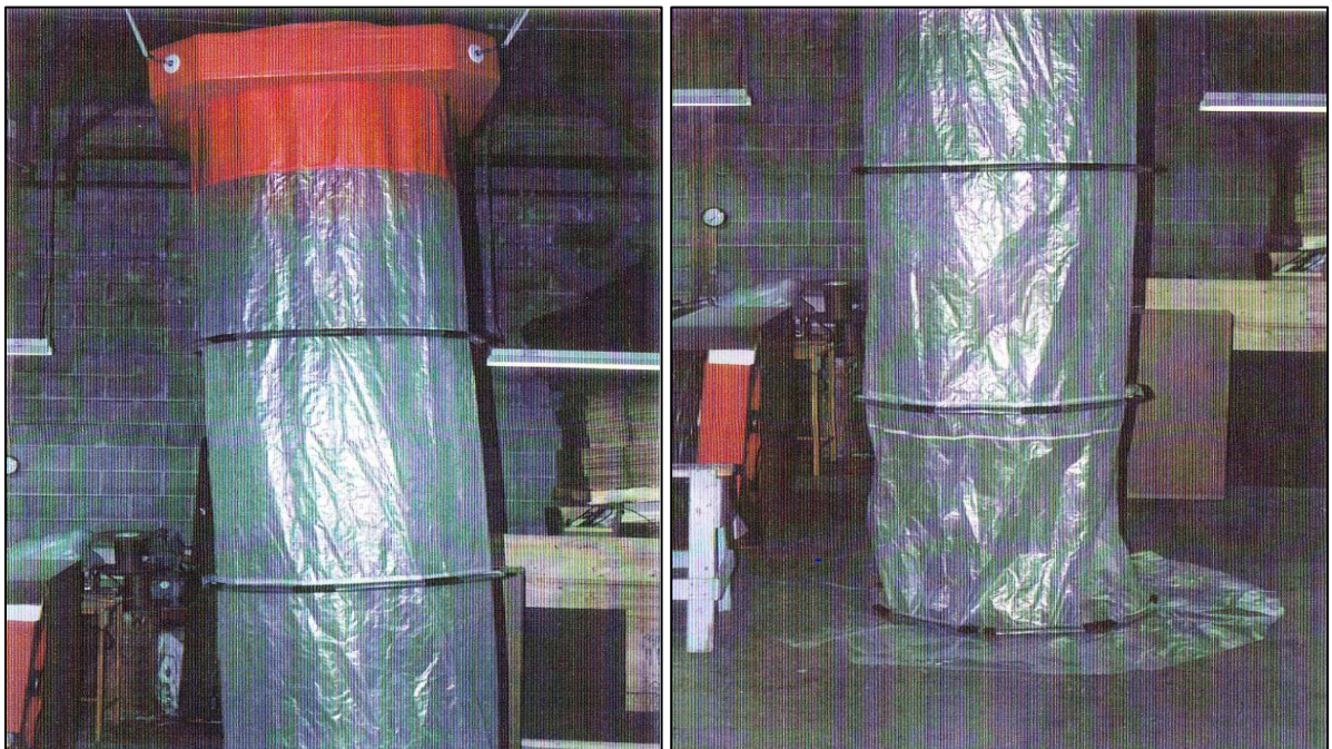
Figure B-4: Limnocorral with lake divider curtains. Poly-pipe rings in belt loop pockets with anchoring skirt provide stability and reduce leakage (Curry Industries 2016).
