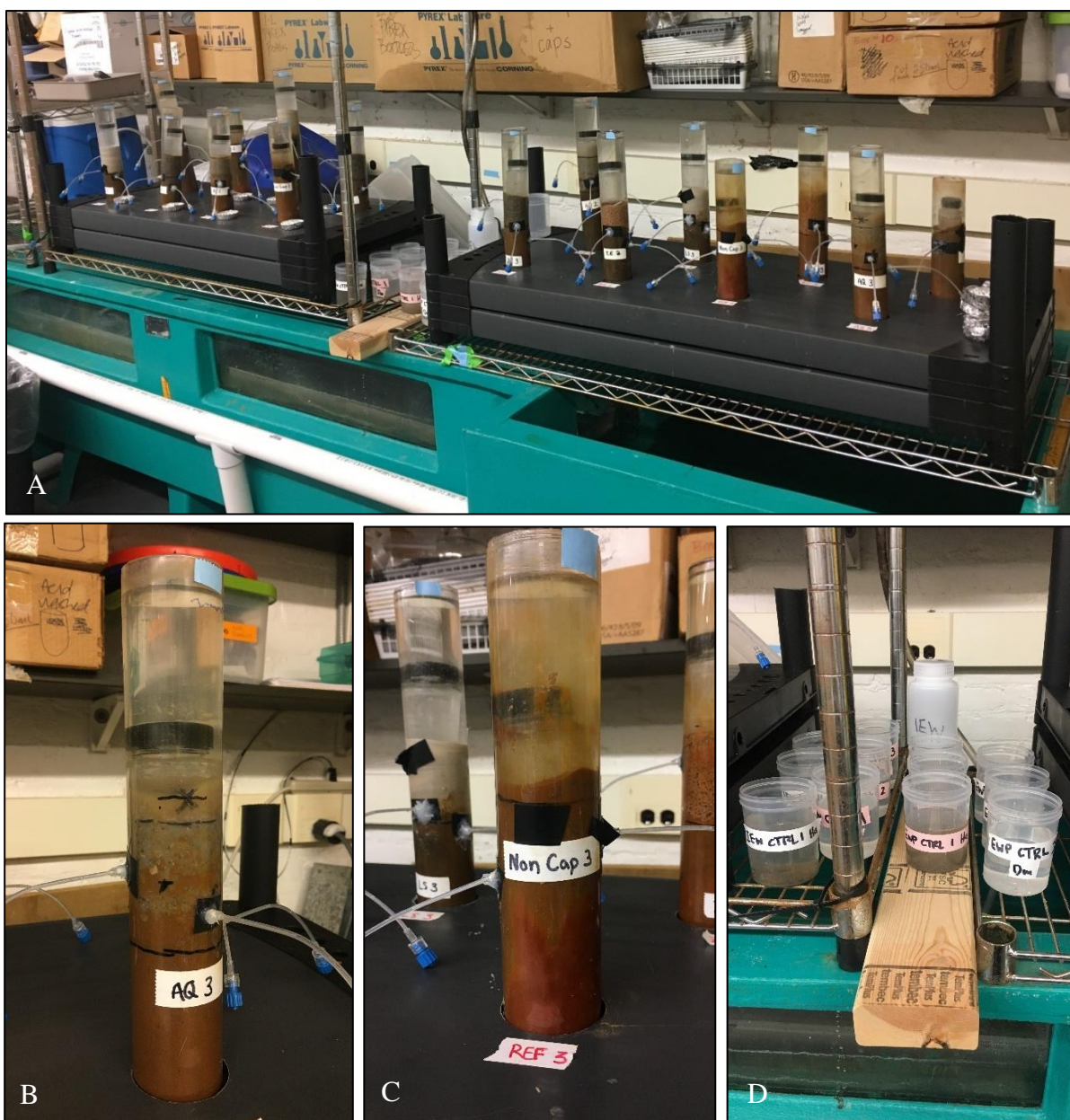
Figure B-8: Task 3 laboratory study setup where A) Overall setup, B) Aquablok treatment, C) Non-capped treatment, and D) EWP and IEW controls.
