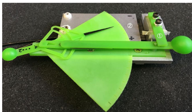
FIGURE 5 Strain amplification sensor with aluminum base on piezo actuator (① Short sensor arm ② Aluminum base)
