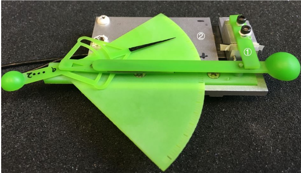
Figure 6: SAS with Aluminum Base on Piezo Actuator (① Short Sensor Arm ② Aluminum Base)
