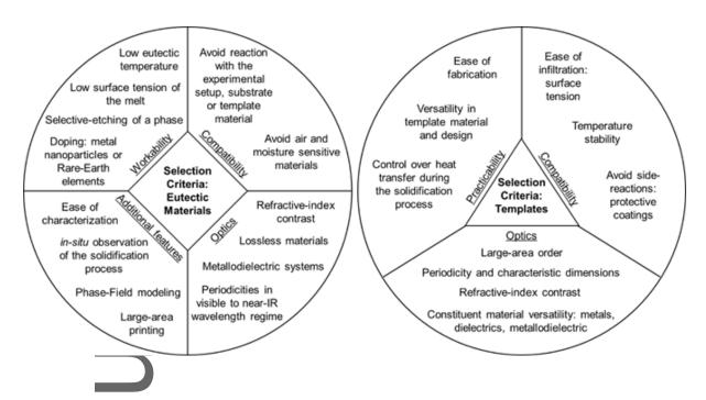
Figure 13. Selection criteria for eutectic materials and templates to obtain structures for optical applications.
