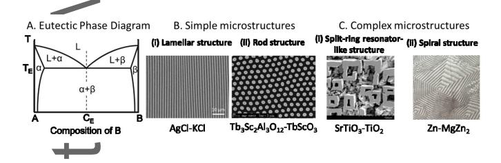
**Figure 4.** Directionally solidified eutectics. A) Schematic of a typical binary eutectic phase diagram. Examples of simple microstructures: B-(i) Lamellar structure (AgCl-KCl eutectic) and B-(ii) Rod
