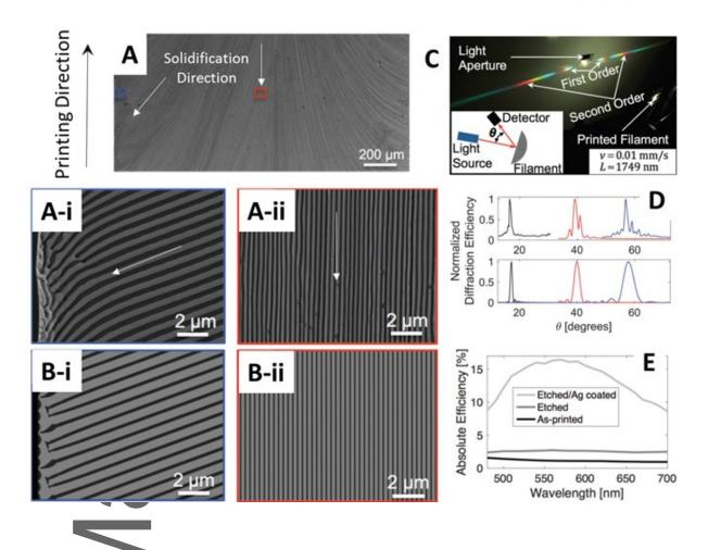
**Figure 7.** Printed eutectic filaments as diffraction gratings: AgCl–KCl eutectic printed using the direct-ink-writing technique. The center of the printed filament shows straight lamellae aligned along the printing direction. At the edges of the filament, the lamellae curve outwards as confirmed by the phase-field modelling. Reproduced with permission. [94] Copyright 2016, Wiley-VCH.
