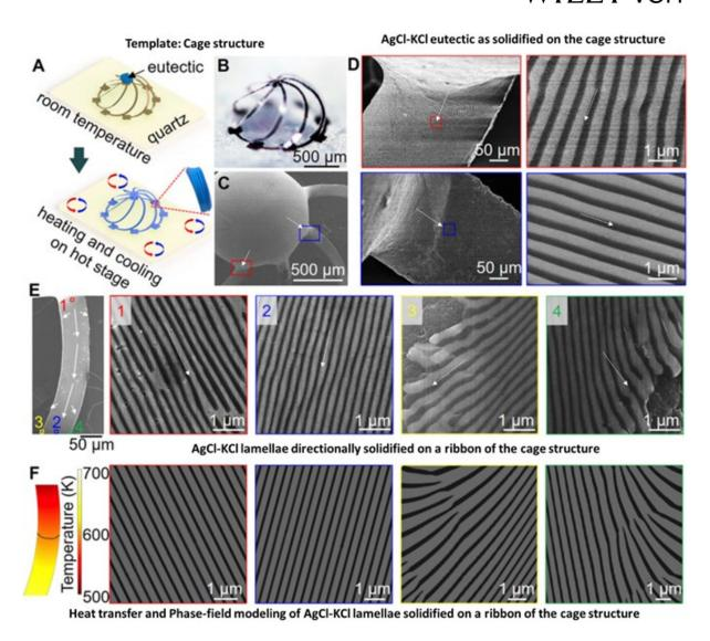
**Figure 8.** Three-dimensional cage structure template-directed solidification of eutectic: AgCl–KCl eutectic as solidified on a cage structure. Reproduced under the terms of the CC-BY-NC-ND 4.0 license. [194]
