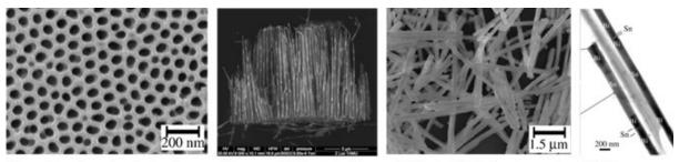
Template: Anodized-aluminum oxide Bi-Sn eutectic as solidified within the channels of AAO
