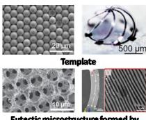
Eutectic microstructure formed by template-directed solidification
