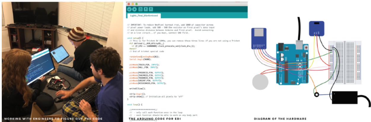
Figure 21. The diagram on the far right represents the connections between all of the electronic components. The middle image is a snippet of the Arduino code. I worked with my engineer friends to bridge the hardware and software
