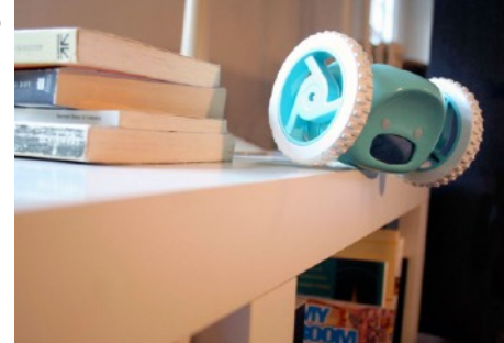
Figure 4. Using its wheels, Clocky rolls off the nightstand, and all around the floor, essentially running away from the user.
