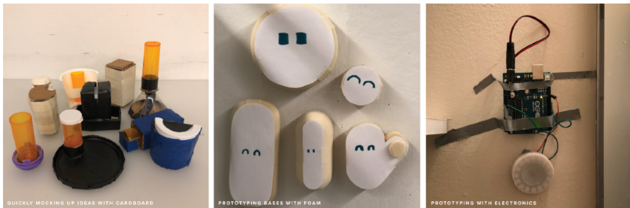
Figure 14. I prototyped forms with scrap materials and foam. I also prototyped interactions using Arduino and neopixels.
