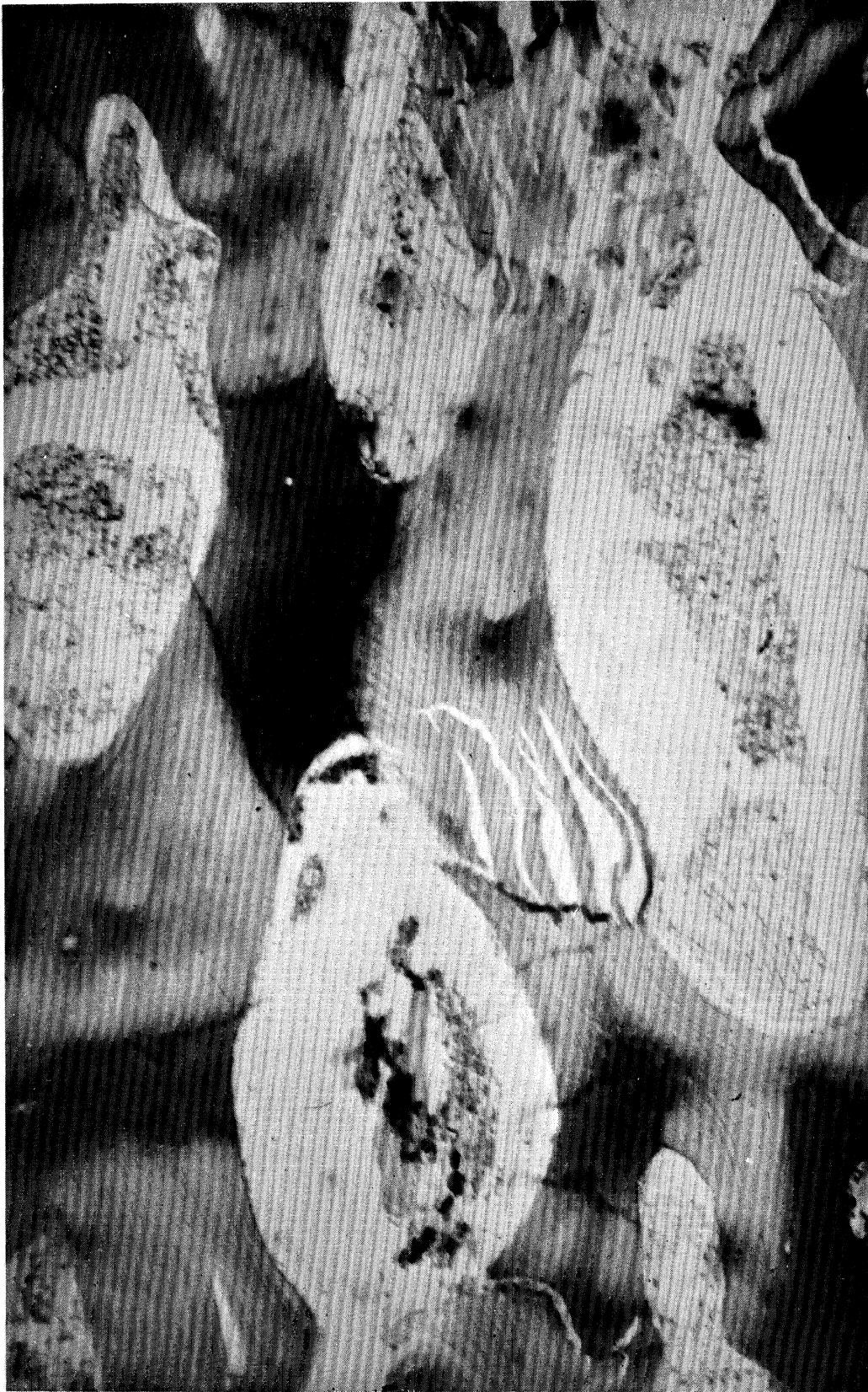
Figure 12 Photomicrograph of Failed Trabeculae of a Diplolæ Layer Compression Specimen (40X)
