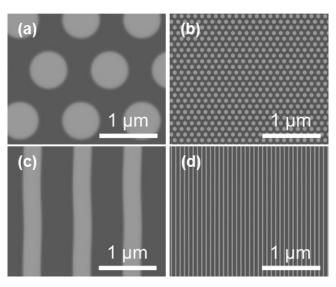
Figure 6. Phase field simulation of directional solidification for (a) v = 0.01 mm/s with rod initial condition, (b) v = 0.53 mm/s with rod initial condition, (c) v = 0.01 mm/s with mixed initial condition, and (d) v = 5.3 mm/s with mixed initial condition. Light gray and dark gray represent AgCl and
