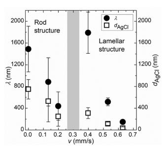
Figure 2.  $\lambda$  and  $d_{AgCl}$  plotted as a function of draw rate v. Here, error bars represent  $\pm 2$  standard deviations. Shaded region corresponds to the observed mixed structure regime.
