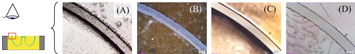
Figure 3.24: Optical micrographs of typical rim conditions observed after lapping and CMP of BB resonator rims that are supported by the various thermoplastics shown in Figure 3.23.
