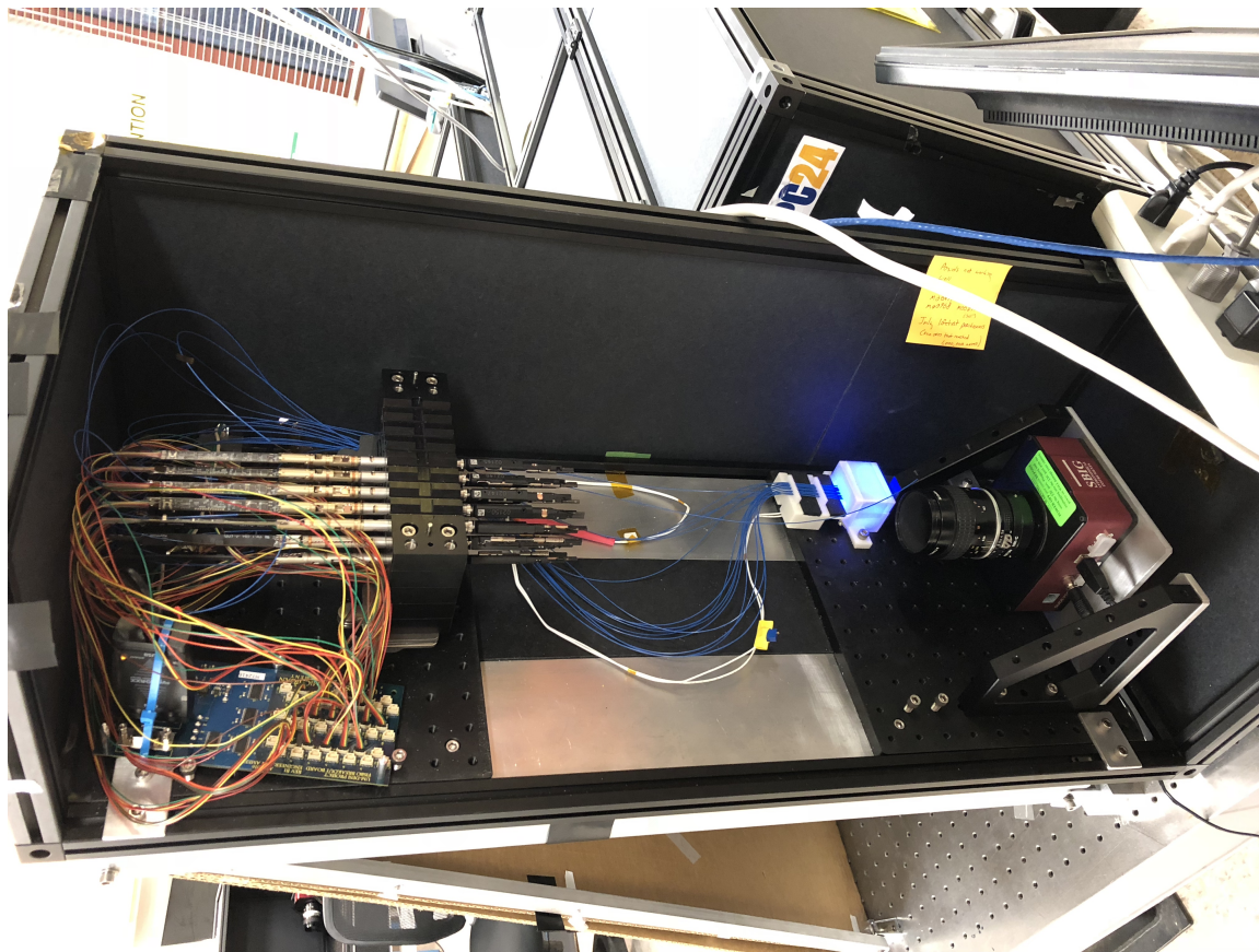
Figure 2.2: One of the test stands used for the quality control tests of DESI positioners sent from a BeagleBone Black running with a DESI-specific operating system. This is powered externally and communicates through the university’s network with a PC neighboring the test stand. This PC is also connected by USB to the camera for readout. The camera, block, illuminator, and breakout board are enclosed by panneling in an aluminum frame, which provides the darkness needed for the camera to accurately capture the fiber positions.
