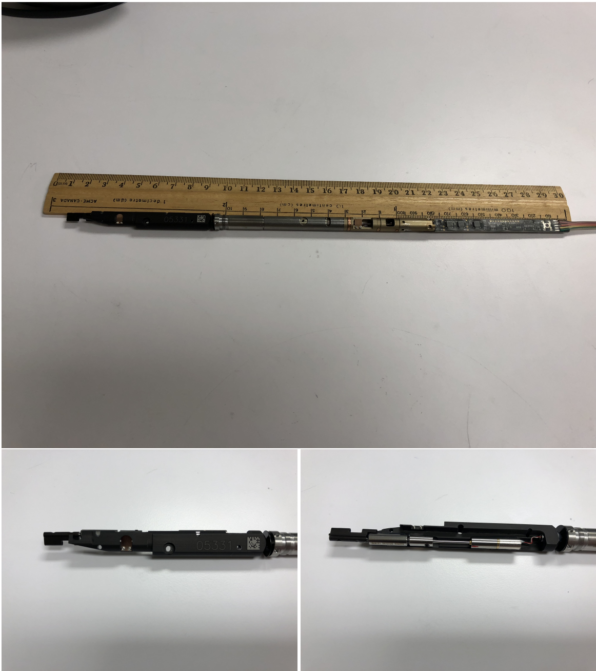
Figure 2.1: One of the positioners that has been produced for use on DESI. Both a full depiction for scale and a closer view of both sides of the upper housing are provided.
