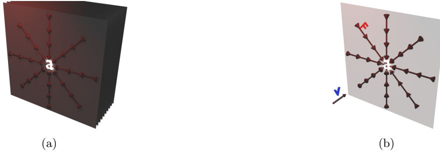
Figure 4: (a) represents a plane central force field imposed on each leaf of a foliation of space. (b) represents an orientation of a vector \mathbf{v} relative to a leaf such that it points to the center a of the central force field at a normal direction. The problem is to express \mathbf{F} pointing towards the center a in terms of \mathbf{v} .
