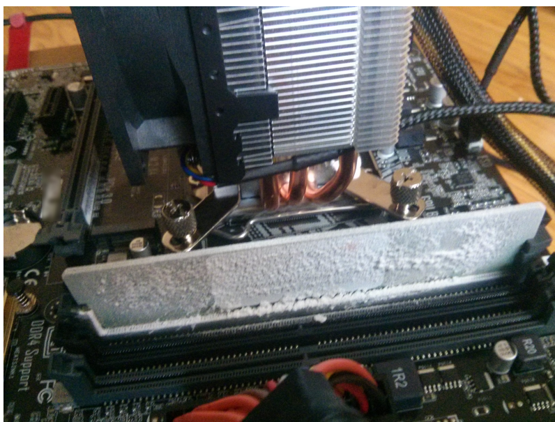
Figure 3.4 Cold Boot Attack on DDR4 DRAM. This photo shows the DRAM in one of our DDR4-based systems. The DRAM is filled with data scrambled by the memory interface of an Intel Skylake-based CPU. The memory has been cooled to -25^{\circ}\text{C} , and it will next be moved to a separate system where its contents will be descrambled.
