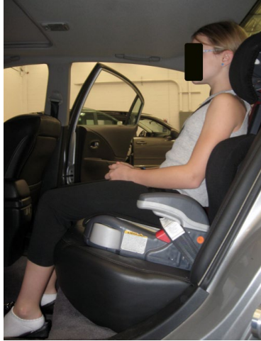
Figure 25. An 11YO participant with stature 1400 mm seated in Nissan Altima with and without a booster.
