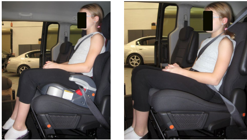
Figure 24. An 11YO subject, stature 1400 mm, seated in Dodge Caravan with and without a booster.
