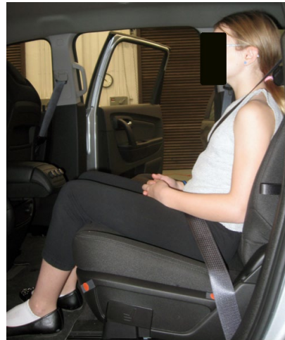
Figure 26. An 11YO subject with stature 1400 mm seated in Chevy Traverse with and without a booster.
