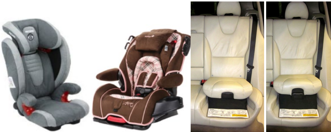
Figure 5. Boosters used in Phase II: ProBooster (left), Alpha Omega (left center), Volvo Integrated at the “Low” position (right center), and the Volvo Integrated at the “High” position (right).
