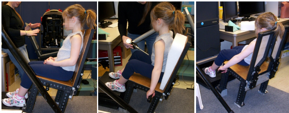
Figure 9. Measuring body landmark locations in the hardseat.
