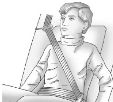
Figure 3. Traverse has an add-on “comfort guide” for the rear seat positions, which is a piece of elastic from the pillar to a plastic sleeve that the shoulder belt slides through.
