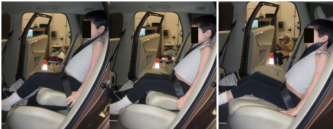
Figure 28. 6YO subject with stature 1131 seated in Volvo with the integrated booster in the high, low, and stowed positions.
