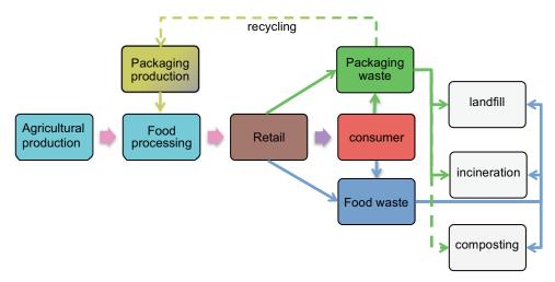
**Figure 1** System diagram indicating the life cycle stages to be included in this study. Thick arrows represent tages where transport is included. Colors correspond to those in figure 3 and figure S1 in supporting information S1 on the Web.
