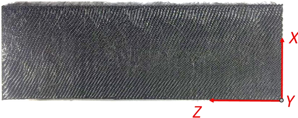
Figure 2.8. Side-view of layer-to-layer specimen (Experiment 7) with surface beading and pitting imperfections due to temperature accumulation during print. These surface imperfections lead to stress concentrations that affect prediction of load capacity. Layers are stacked from right to left.
