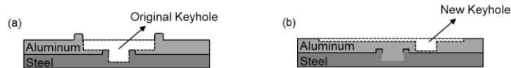
Figure 4-4. Schematic illustration of the weld cross section of the keyhole refilled FSSW
