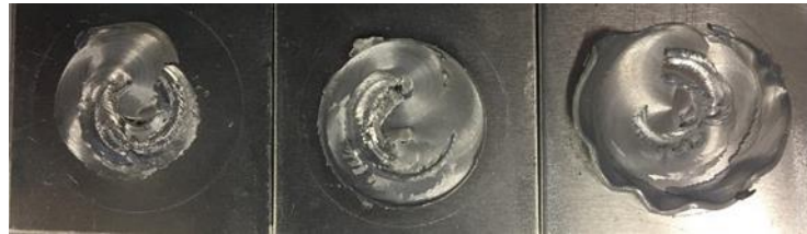
Figure 6-2 Illustrations of keyhole refilled FSSW with spiral retreat configuration
