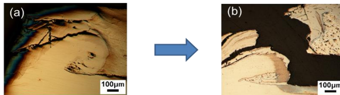
Figure 2-20. Cross section view of the fracture: (a) At the beginning of tensile test: Cracks formed in the IMCs, (b) At the end of tensile test: Cracks propagate and fracture occurs
