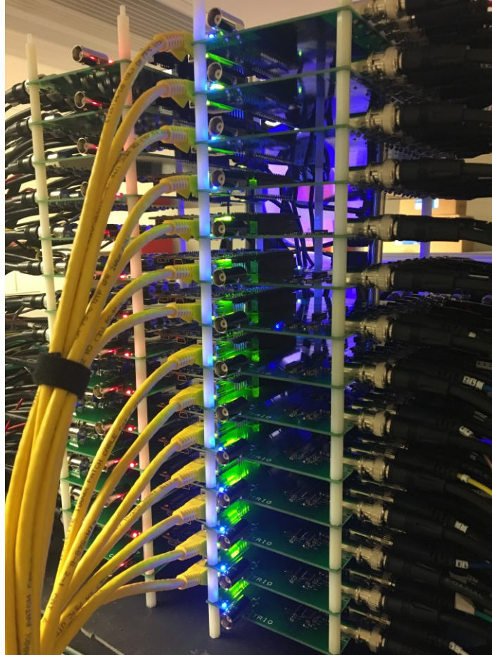
Figure 3.4: The Retrofit System integrated with a 112-channel, 500-kHz histotripsy array. Input data to the receive system is transmitted via the black BNC cables on the left and right sides of the system, and data transmission between the FPGA/SoC modules and the master computer occurs via the yellow Ethernet cables in the middle.
