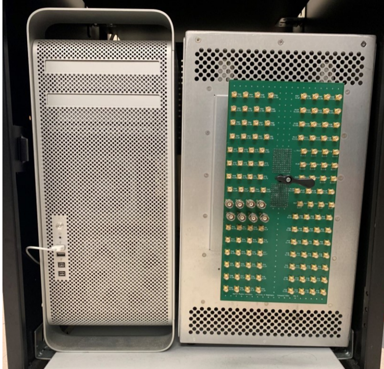
Figure 3.2: Verasonics receive-system prototype including the 128-channel breakout board (right) connected to the standard 128-channel ultrasound connector on the Verasonics transmit-and-receive system.
