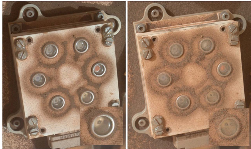
Figure 1. Dust deposition on the ultraviolet sensor: comparison between Mars Science Laboratory sols 2036 (prestorm) and 2216 (after the storm), taken by Mars Hand Lens Imager. The images were taken at different times of sol, hence with different sun position, as evidenced by the different sun glint locations at the edges of the photodiodes. It can be seen in the zooms for both images of the same photodiode that the sensor is almost blocked by the dust, which highlights the deposition of dust over the rover due to the dust storm.
