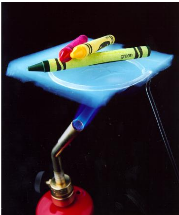
Figure 3.10: Extremely low thermal conductivity of silica aerogel [70].
