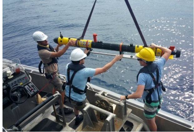
(b) Deployment of the Deep Robot Optical Perception Laboratory (DROP) Lab's Iver autonomous underwater vehicle (AUV) during a research cruise aboard the R/V Falkor .
