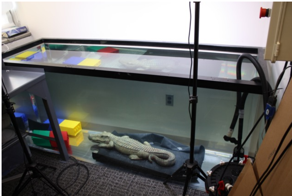
Figure 4.12: Laboratory water tank setup and target object for reconstruction. Lighting and water clarity can be tightly controlled enabling us to test the limits of the proposed approach.
