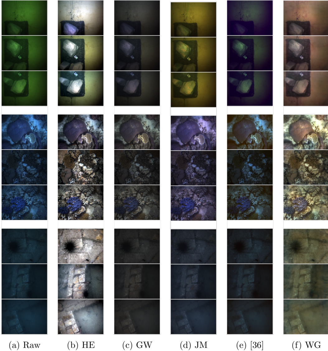
Figure 2.5: Results showing color correction on the Marine Hydrodynamics Laboratory (MHL), Lizard Island, and Port Royal datasets (from top to bottom). Each column shows (a) raw underwater images, and corrected images using (b) histogram equalization (HE), (c) normalization with the gray world assumption (GW), (d) a modified Jaffe-McGlamery model (Eqn. 3) with ideal attenuation coefficients (JM), (e) Shin et al.’s deep learning approach ([36]), and (f) WaterGAN (WG).
