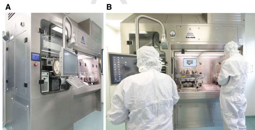
Figure 29. Custom-made GMP-compliant flow cytometric cell sorter (A) with auxiliary equipment cabinet (left) and laminar air flow hood (right) containing the sort chamber and (B) the sort unit in operation (safety-cabinet-enclosed sort unit seen between the two operators).
