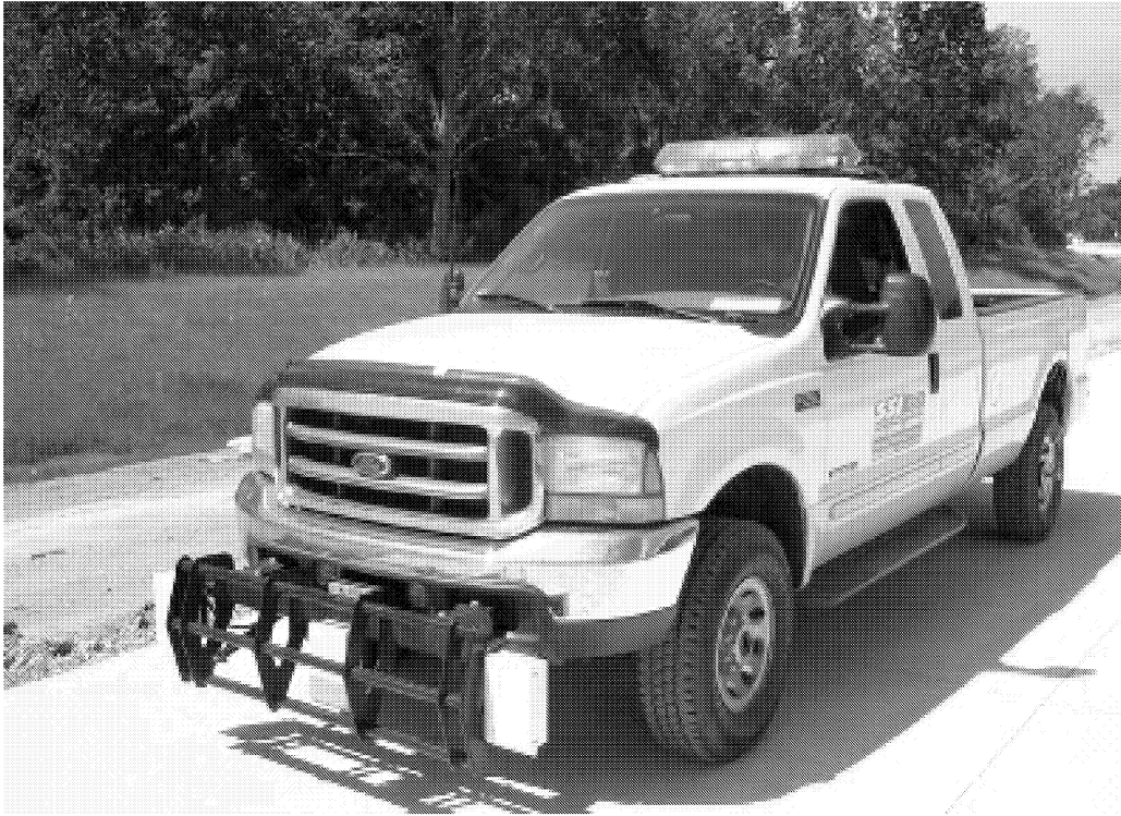
Surface Systems Instruments High-Speed Profiler at Site 4.
