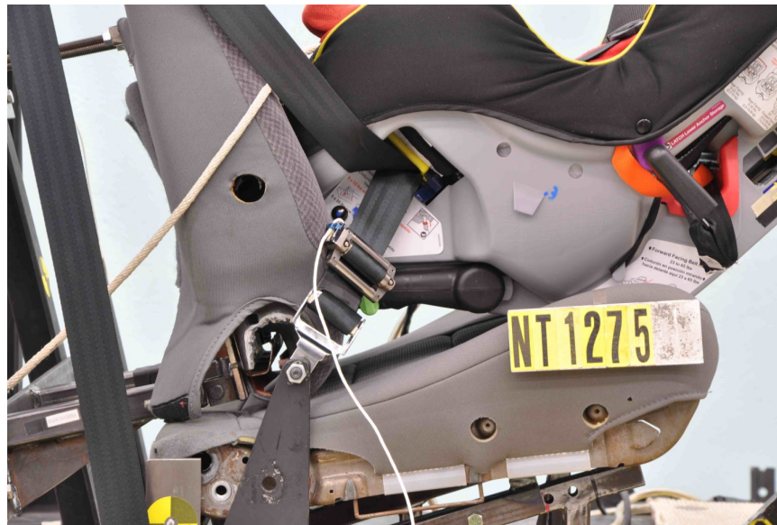
Figure 23. Child restraint installed with gap to achieve same initial angle achieved under FMVSS No. 213 conditions
