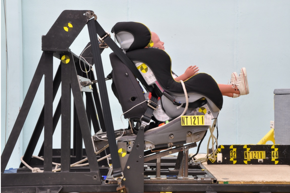
Figure 9. Pretest photo of TrueFit test with FMVSS No. 213 belt geometry and 350-mm cushion length
