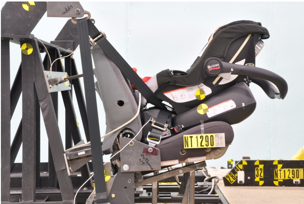
Figure 10. Pretest photo of Britax Chaperone tested with 400-mm cushion length and 6YO-Optimal belt locations
