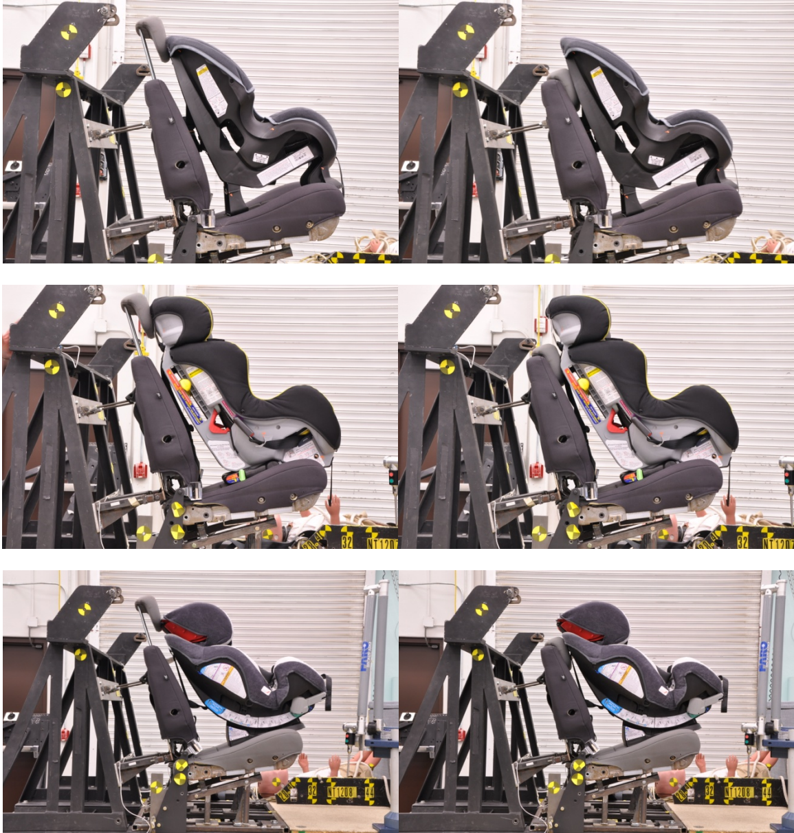
Figure 12. Head restraint interfered with child restraint installation in both the full up (left column) and full down (right column) positions
