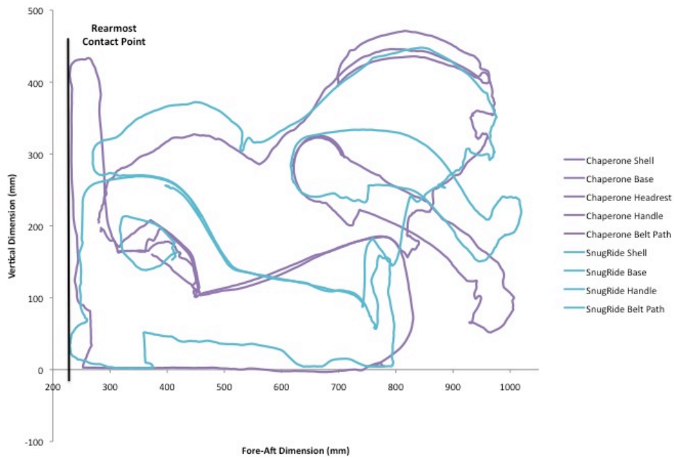
Figure 6. Right-side profile and belt paths of rear-facing infant seats with bases
