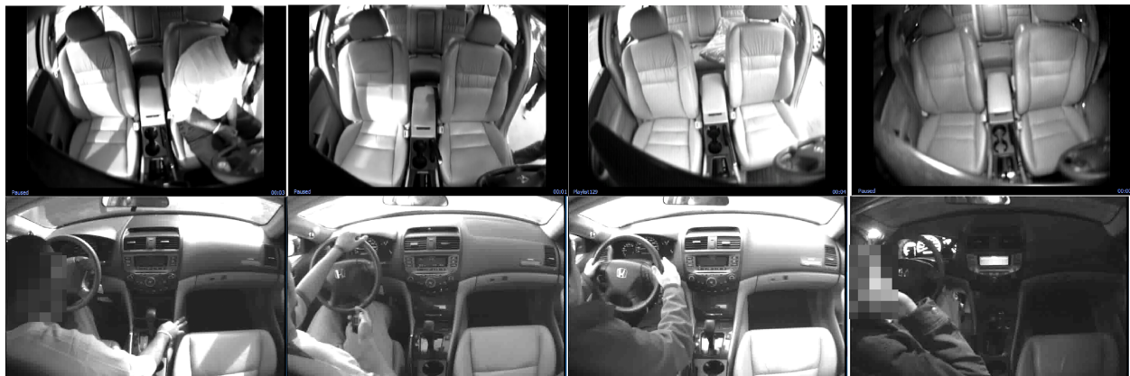
Figure 5. Range of camera views in one vehicle across different drivers. The ceiling camera remained relatively fixed, but the windshield camera moved.
