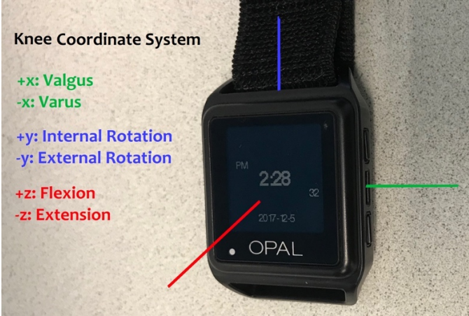
Figure 8 | APDM Opal's appearance and coordinate system
