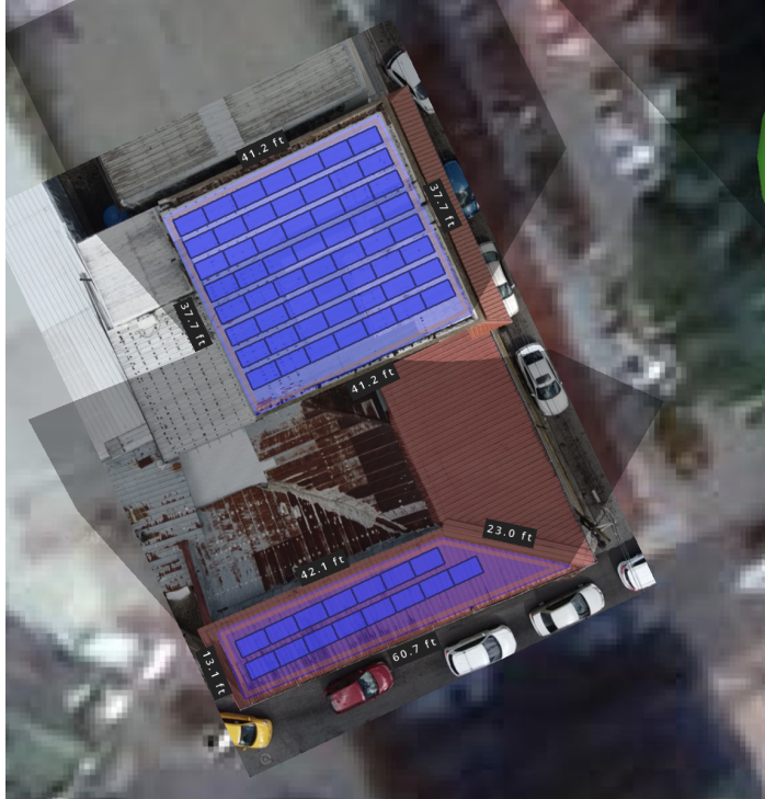
Figure 11: Overlay on Lucy's Pizza and the Flush Mountain Racking for its tilted roof.
