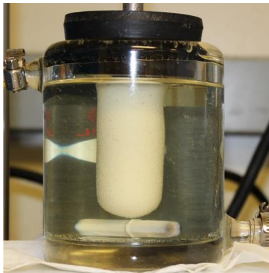
Figure 2-5: A wax deposit forming on a cold finger
