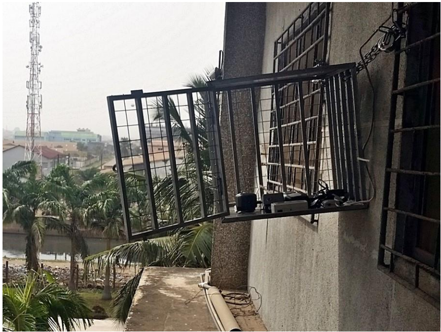
64 Figure S4. Photo of sampling cage with monitoring instruments mounted on building at site 3.
