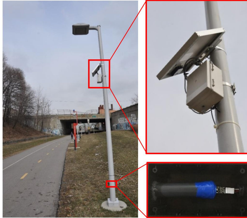
Figure 6-9. Urbano sensing node measuring pedestrian traffic along the Dequindre Cut in Detroit, MI.
