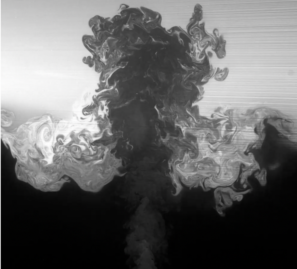
The refractive-index matched turbulent jet penetrating a sharp density interface.
