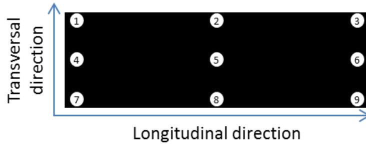
Figure 3.2 Top view of the CFRP workpiece: Showing the locations of the nine samples cut from the workpiece and used for DSC
