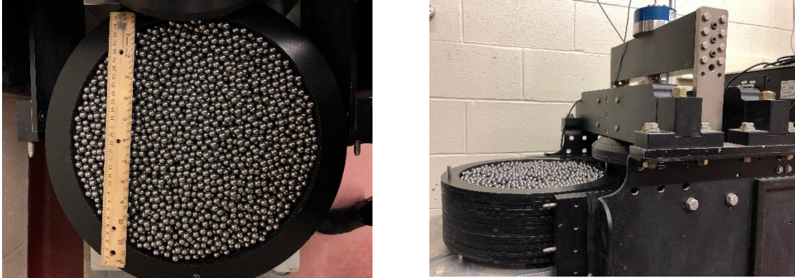
Figure 3.3 Prepared specimen of uniform-sized chrome steel sphere
