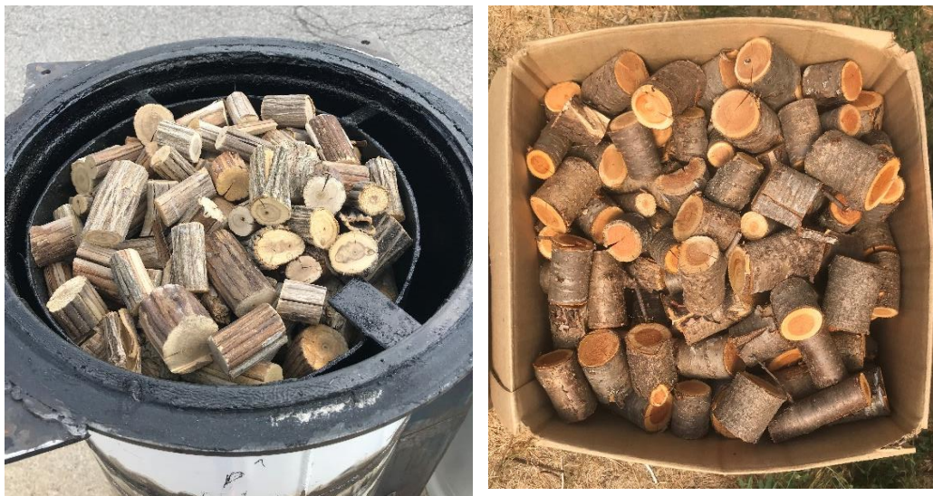
Fig. 2. Samples of dry, cut honeysuckle (left) and buckthorn (right) used as feedstock for gasification trials.
