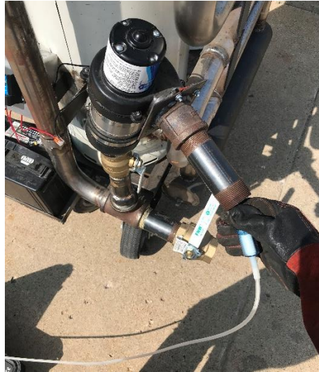
Fig. 4. Set up for collecting data on the composition of the produced syngas.
